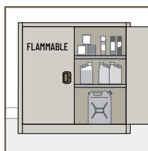
2 Flammable products stored securely away from house in locked cabinets with latches.
