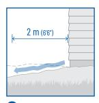
Correct grading to direct water at least 2 m away from foundation.
