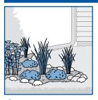
Install a rain garden to collect stormwater (at least 5 m from the foundation).
