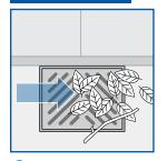
1 Remove debris from nearest storm drain or ditch and culvert.
