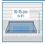
Install window wells that sit 10-15 cm above ground, and window well covers (where fire escape requirements permit).
